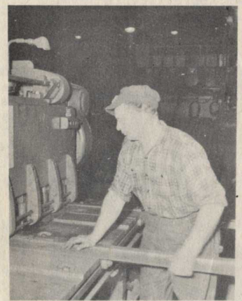
HERBERT BENNETT cuts steel on power shear.
